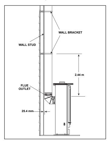
Figure 10.12 Installing Support Brackets
